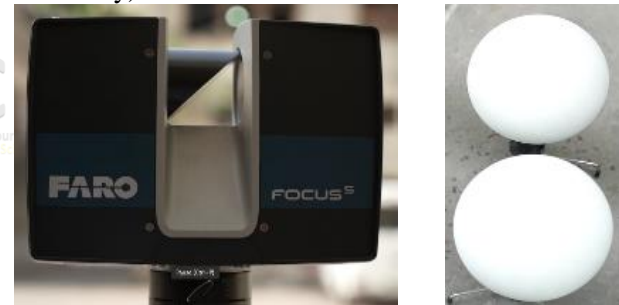
Figure 8: Faro Focus s (TLS) (Left )and Spheres (Targets) (Right) (Source: WCLA)
