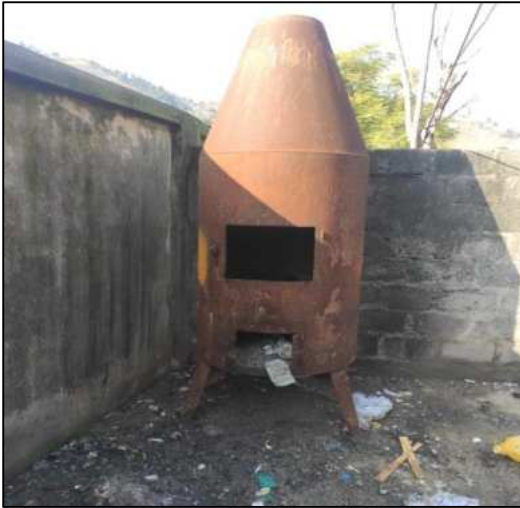
Figure 11 An old rusty burner used for burning sharps used instead of an incinerator
