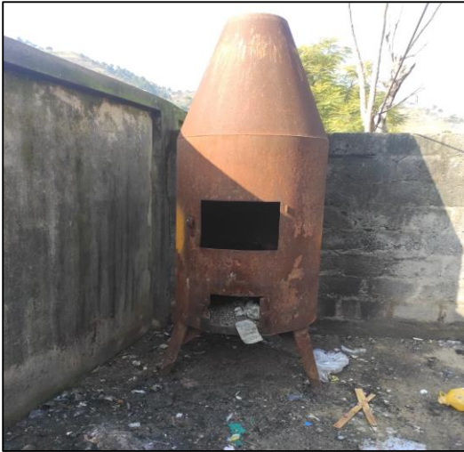
Figure 11 An old rusty burner used for burning sharps used instead of an incinerator
